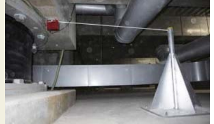
Displacement of the base isolation layer : Displacement gauge (with a stretched string)
