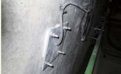
Earth pressure : Earth pressure gauge (in contact with the earth on the outside of the wall)
