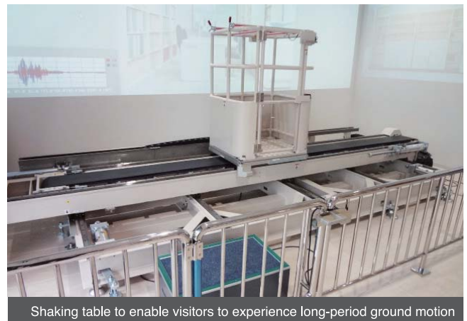
Shaking table to enable visitors to experience long-period ground motion
